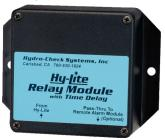
The Relay Module allows the Hy-Lite to perform as a controller of valves, custom alarm systems, etc. The SPDT relay features an adjustable time delay to compensate for expected equipment rinse-up times. There is also a signal pass-thru feature permitting the relay module to be used with the remote alarm module.
