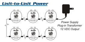
Up to 6 Hy-Lites can be plugged into each other greatly reducing congestion at the wall outlet. The results are a more professional installation! Operational power is a safe 12 VDC supplied by a plug-in style transformer.
